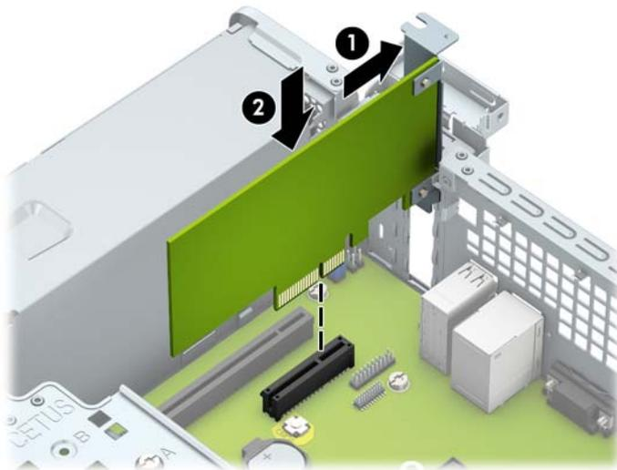
**NOTE:** When installing an expansion card, press firmly on the card so that the whole connector seats properly in the expansion card socket.
