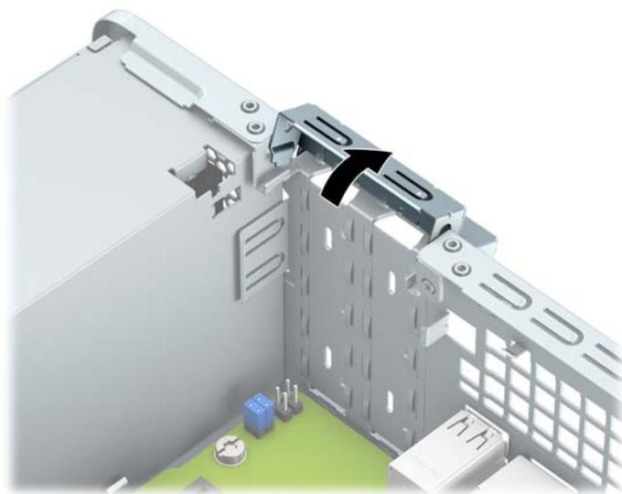
8. Before installing an expansion card, remove the expansion slot cover or the existing expansion card.
