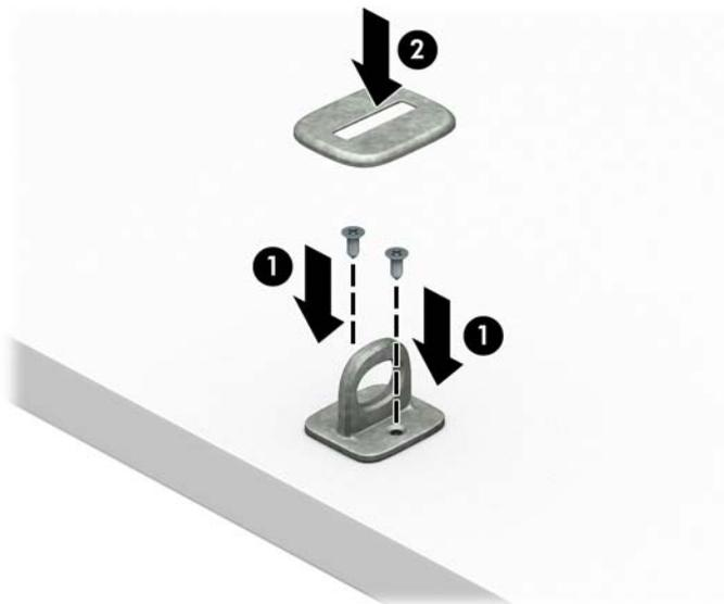
3. Slide the security cable through the security cable fastener.
