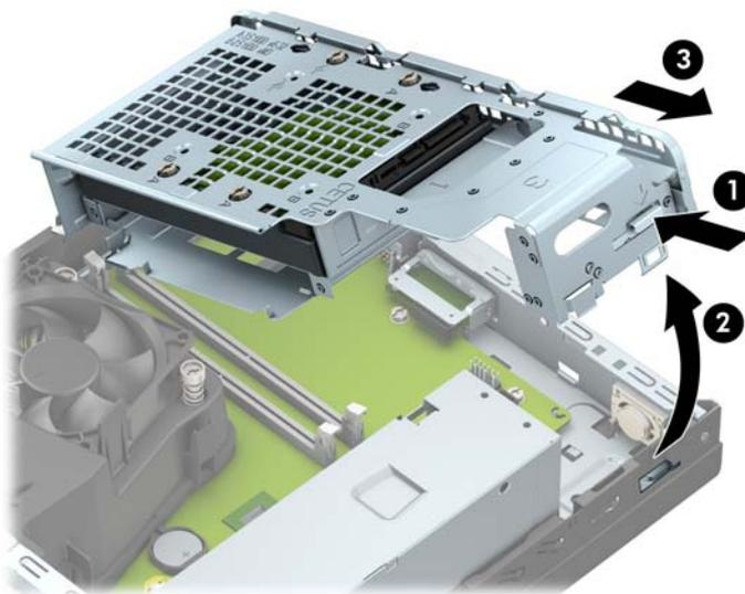
10. Remove the hard drive from the drive cage.
