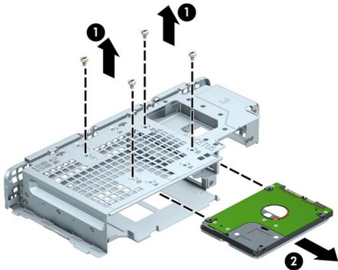
**11.** Install the new drive in the drive cage.
