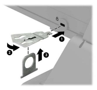
Slide the security cable through the security guide installed on the monitor.
