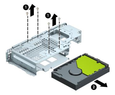
• If you are removing a 2.5-inch hard drive, remove the four screws that secure the drive to the drive cage (1) to release the drive (2).
