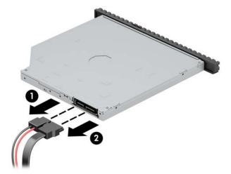
7. Press the release lever on the back of the drive (1), and then slide the drive through the front bezel (2).
