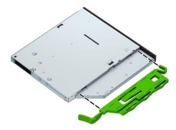
8. Slide the optical drive through the front bezel all the way into the bay (1) so that it locks in place (2).
