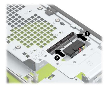
14. Slide the optical drive through the front bezel all the way into the bay (1) so that it locks in place (2).
