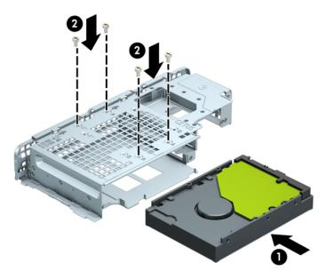
• If you are installing a 2.5-inch hard drive, slide the drive into the drive cage (1) and secure the drive with four M3 metric screws.
