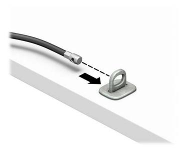
4. If your workstation configuration includes a monitor that you want to secure, pull the two scissor hands of the monitor lock apart and insert the lock into the security slot on the rear of the monitor (1), close the scissor hands together to secure the lock in place (2), and then slide the cable guide through the center of the monitor lock (3).
