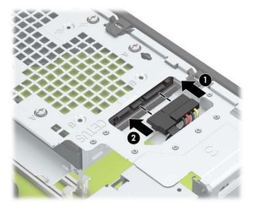
13. Slide the optical drive through the front bezel all the way into the bay (1) so that it locks in place (2).
