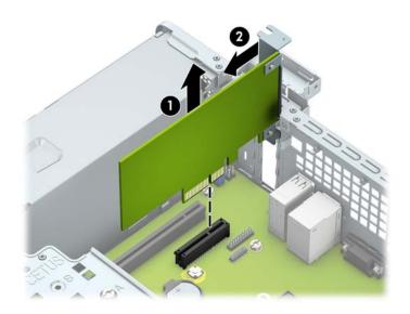
c. If you are removing a PCI Express x16 card, pull the retention arm on the back of the expansion socket away from the card and carefully rock the card back and forth until the connectors pull free from the socket. Pull the expansion card straight up from the socket.
