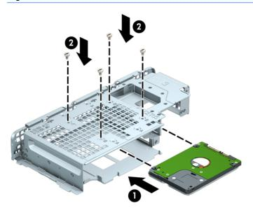
12. Hold the drive cage at an angle and insert the tabs on the side of the drive cage into the slots on the chassis (1), and then lower the other side of the drive cage down so that the latch snaps onto the chassis (2).
