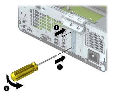
**b.** If you are removing a PCI Express x1 card, hold the card at each end, and carefully rock it back and forth until the connectors pull free from the socket. Pull the expansion card straight up from the socket (1), then remove the card from the expansion slot cover tray (2).
