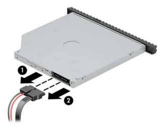
Press the release lever on the back of the drive (1), and then slide the drive through the front bezel (2). **7.**
