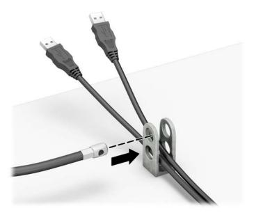
8. Remove the thumbscrew from the rear of the chassis and screw the lock to the chassis in the thumbscrew hole. Insert the plug end of the security cable into the lock (1) and push the button in (2) to engage the lock. Use the key provided to disengage the lock.
