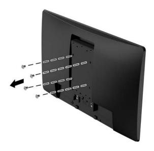
4. Secure the mounting plate to the wall or swing arm of your choice using the four screws included with the mounting plate.
