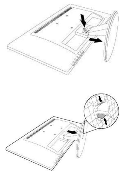
**Note:** The monitor supports the VESA industry standard 100mm mounting holes. To attach the display head to a wall, swing arm or other mounting fixture, follow the manufacturer's mounting instructions. For the best performance, use the power and video cables provided with the monitor.
