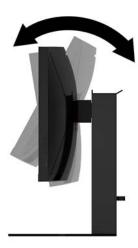
Adjust the display head up or down to set it to a comfortable eye level.
