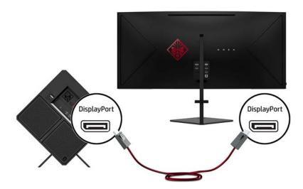
3. Connect one end of a Mini DisplayPort cable to the DisplayPort port on the rear of the monitor and the other end to the Mini DisplayPort port on the source device (cable not provided).
