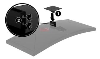
3. To attach the display head to a swing arm or other mounting device, insert four mounting screws through the holes on the mounting device and into the screw holes on the VESA mounting bracket.
