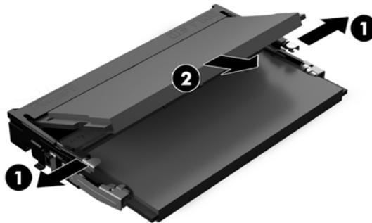
6. Slide the new memory module into the slot at approximately a 30° angle (1), then press the memory module down (2) so that the latches lock it in place.
