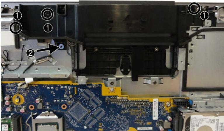
7. Remove the webcam shield from the computer.
