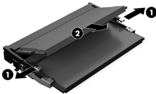
4. Slide the new memory module into the slot at approximately a 30° angle (1), then press the memory module down (2) so that the latches lock it in place.
