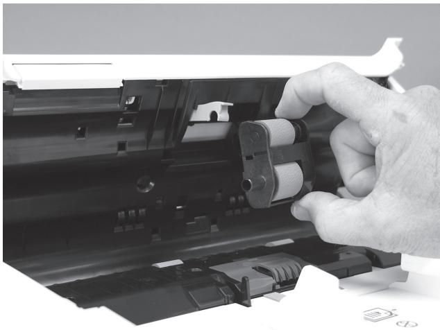
**EN** **NOTE:** The two short drive shafts face the rear of the document feeder. The single long shaft faces the front of the document feeder.
