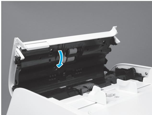
**EN** **NOTE:** If the latch interferes with the roller assembly, make sure that the roller assembly drive shafts are completely seated in the holder.
