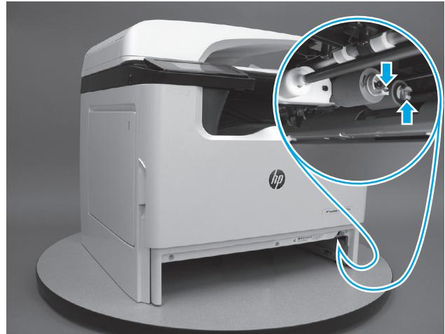
**EN** **A4 dual Tray 2/3 and A3 single Tray 2 pickup and feed rollers install:** Squeeze the locking tab on a roller, and then slide the roller all of the way onto the shaft.
