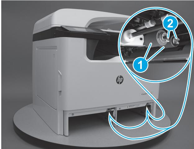
**EN** **Pickup and feed roller removal:** Look up into the tray cavity, and locate pickup and feed rollers (callout 1). Squeeze the locking tab on a roller (callout 2), and then slide the roller off of the shaft.
