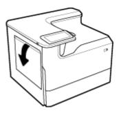
2. According to the media mark on the tray, place envelopes in Tray 1 face-down, with the top of the envelope oriented toward the back of the printer.
