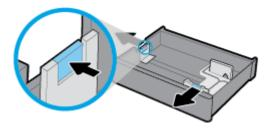
3. Place the paper in the tray and make sure that it is flat at all four corners. Close the length and width paper guides against the loaded media.
