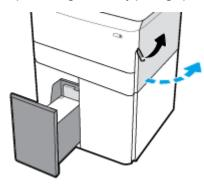
**4.** Open the lower right door, by pushing down on the lower latch.
