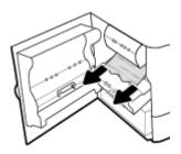
4. Lift up the duplexer, and gently remove any visible paper under it.
