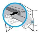
**b.** Slide the left-hand side of the duplexer through the opening in the left rail, and then push the blue latch back into position.
