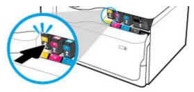
3. Grasp the edge of the old cartridge and then pull the cartridge straight out to remove it.
