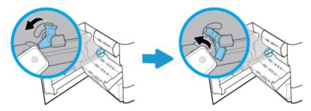
**b.** Pull the right-hand side of the duplexer out of the right rail, and remove the duplexer.
