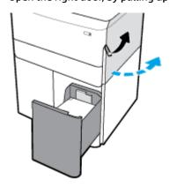
4. Open the lower right door, by pushing down on the lower latch.
