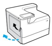
2. Grasp the handle of the duplexer, and pull the duplexer out as far as possible.
