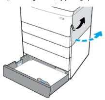
4. Open the lower right door, by pushing down on the lower latch.
