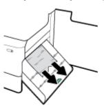
4. Lift up the duplexer, and gently remove any visible paper under it.
