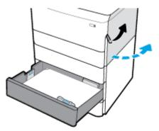
4. Open the lower right door, by pushing down on the lower latch.
