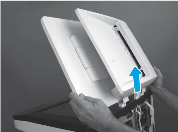
**EN** Open the document feeder, and then lift it straight up until it stops at the retention tab on each hinge.
