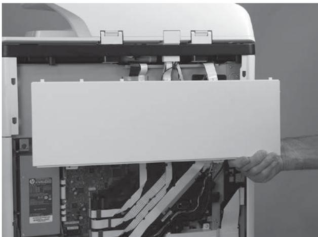
EN Remove the rear cover spacer.
