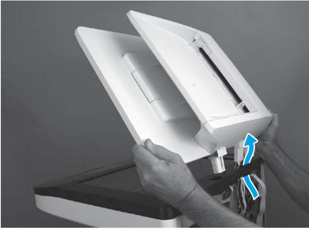
**EN** Carefully thread the document feeder FFCs and ground wire up and through the hole in the scanner cover to remove the document feeder.
