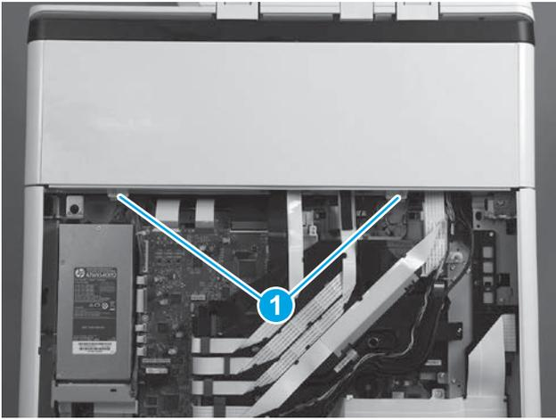
**EN** Remove the rear cover spacer (772zt and 777hc/z only)
