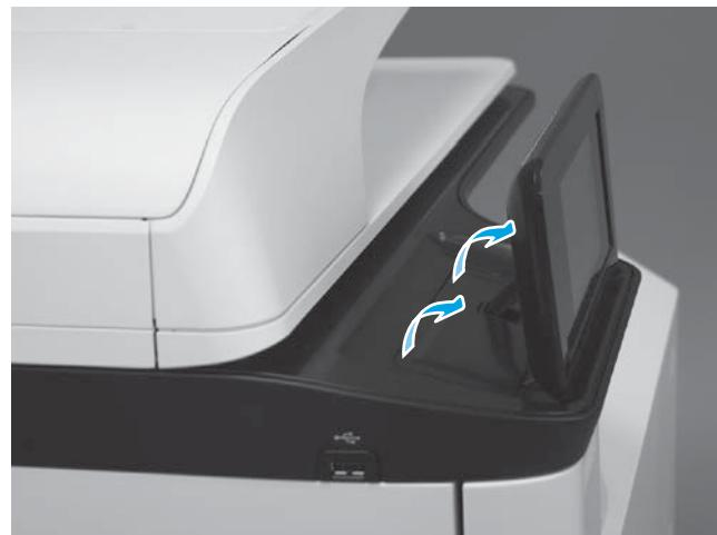
**EN** Use a small flat-blade screwdriver to release two tabs (located along the top edge of the cover), and then remove the cover.
