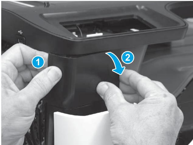
**EN** At the front of the printer, flex the corner of the cover away from the printer (callout 1), and then rotate the top edge away from the printer (callout 2) to remove the cover.
