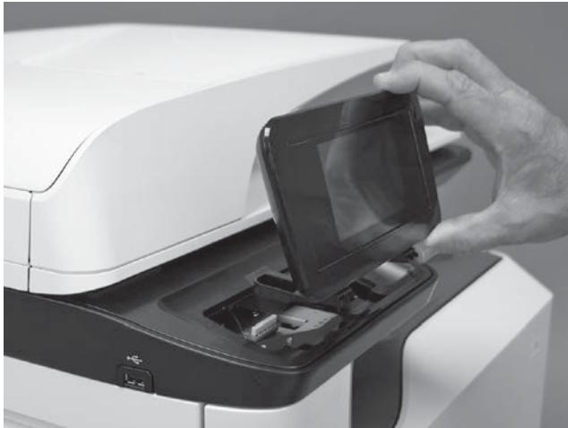
EN Remove the control panel.
