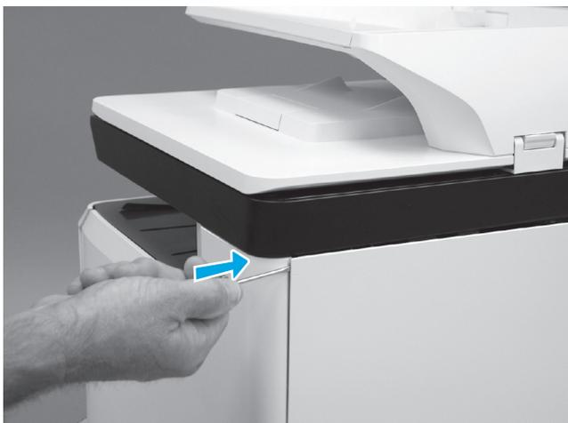
**EN** Use a small flat-blade screwdriver to carefully pry the top left corner of the rear cover away from the printer, and then push in against the latch to release it.
