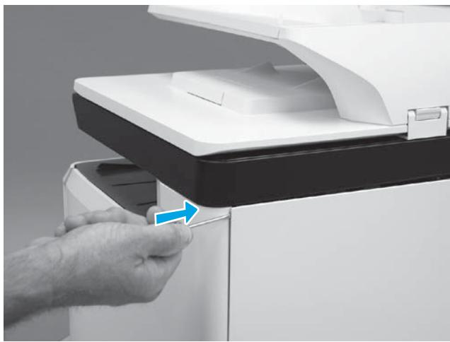
**EN** Use a small flat-blade screwdriver to careful pry the top left corner of the rear cover away from the printer, and then push in against the latch to release it.
