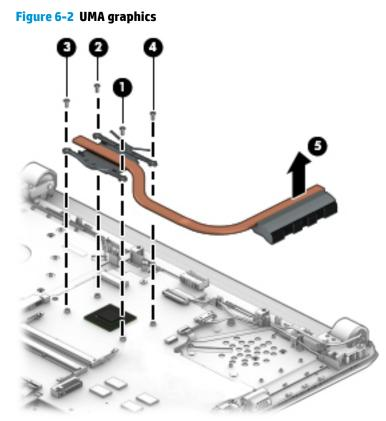
• UMA graphics Thermal paste is used on the heat sink (1) and the processor (2).
