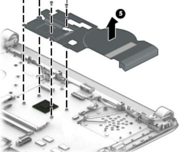
• UMA graphics (fanless) Thermal paste is used on the heat sink (1) and the processor (2).
