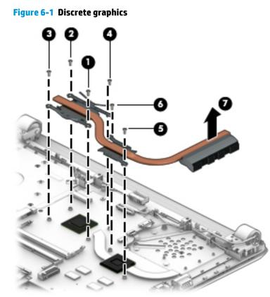
• **Discrete graphics** Thermal paste is used on the processor and associated heat sink area (1)(2), as well as the graphics chip and associated heat sink area (3)(4).
