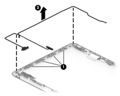
7. Use the following image to determine proper cable routing around the hinges.
