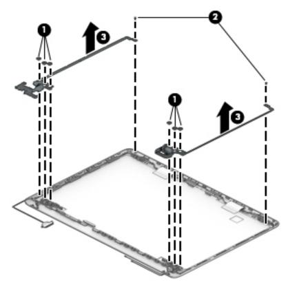
5. To remove the wireless antennas an cables, release the cables from the clips built into the side of the display enclosure (1), and then remove the antennas and cables (2)(3).
