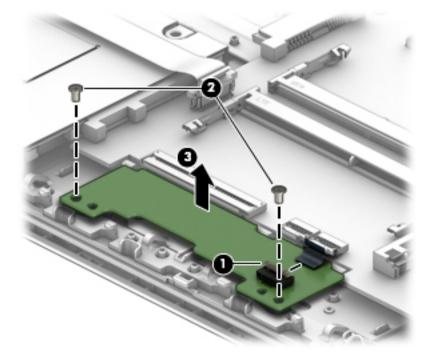
Reverse this procedure to install the TouchPad button board.
