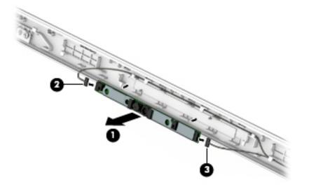
**3.** To remove the infrared (IR) camera/microphone module:
