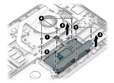
Reverse this procedure to install the TouchPad board.
