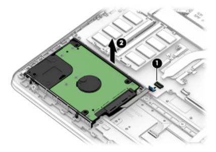
3. To remove the hard drive bracket and connector, pull the connector away from the hard drive (1).
