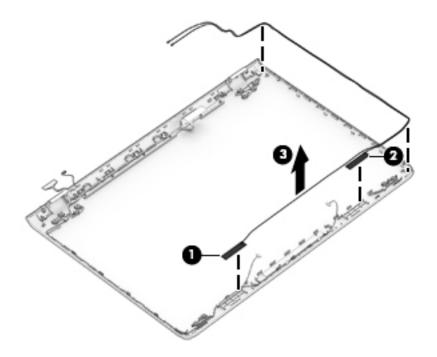
To remove the display/camera cable, disconnect the cable from the board at the bottom of the display (1) and the camera at the top of the display (2), and then remove the cable from the clips built into the side of the display enclosure (3).
