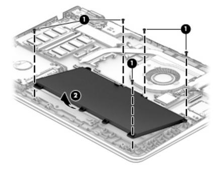
Reverse this procedure to install the battery.
