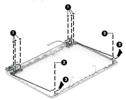
6. To remove the wireless antennas and cables, peel the left(1) and right (2) antennas off the display enclosure, and then remove the antennas and cables from the display enclosure (2).
