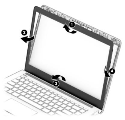
**3.** To remove the standard camera/microphone module:
