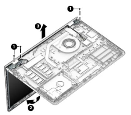
If it is necessary to replace any of the display assembly subcomponents:
