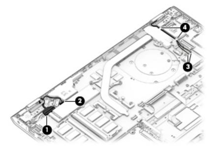
5. Remove the lock bracket from atop the right hinge by removing the Phillips PM2.5×6.0 screw (1) and then lifting the bracket off the hinge (2).
