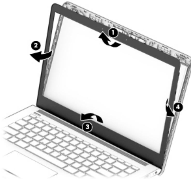
2. To remove the standard camera/microphone module:
