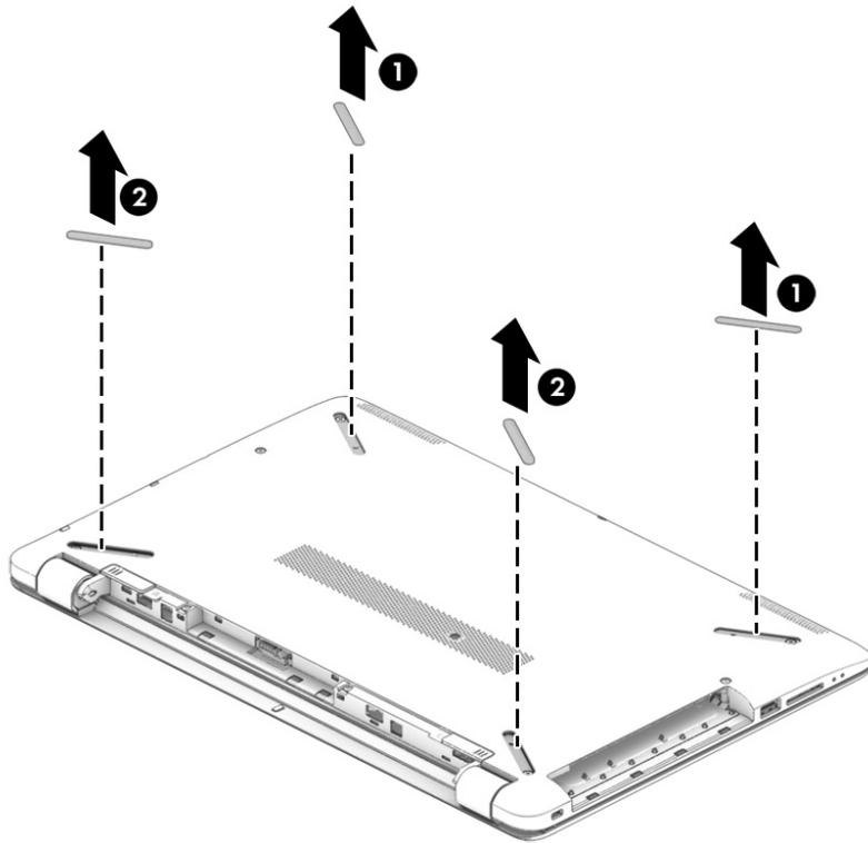
Reverse this procedure to install the rubber feet.
