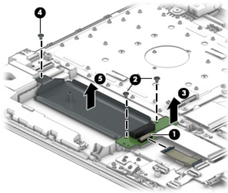
Reverse this procedure to reassemble and install the solid-state drive adapter bracket and connector board.
