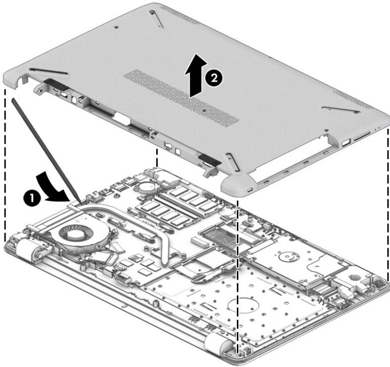
Reverse this procedure to install the bottom cover.
