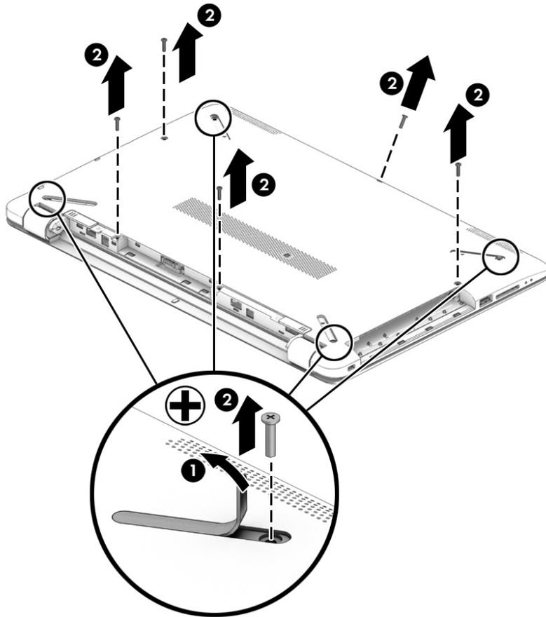
4. Start prying at the front of the computer and work around to the back to separate the bottom cover from computer **(1)**, and then remove the bottom cover **(2)**.
