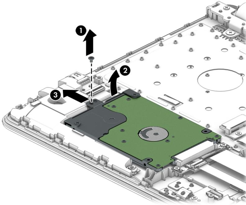
4. To remove the hard drive bracket, remove the two Phillips PM3.0×3.0 screws **(1)** that secure the bracket to the hard drive.
