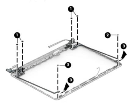
5. To remove the wireless antennas and cables, peel the left(1) and right (2) antennas off the display enclosure, and then remove the antennas and cables from the display enclosure (2).
