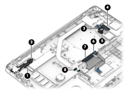
2. Remove the four Phillips PM2.0×5.0 screws (1) that secure the system board to the computer.
