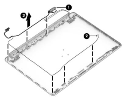
7. If replacing the display enclosure, be sure that the subcomponents (including the camera/microphone module, the antenna receivers, and all associated cables and hardware) are transferred to the new enclosure.
