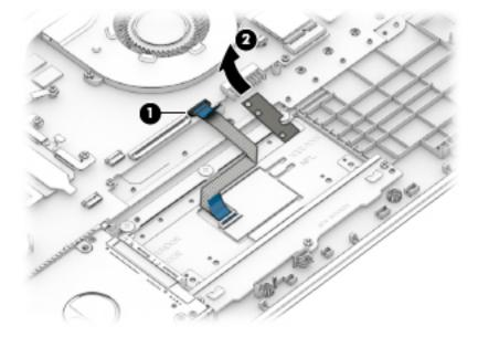
3. Remove the three Phillips PM2.0×3.0 screws (1) that secure the bracket to the computer, and the lift the bracket from atop the TouchPad (2).
