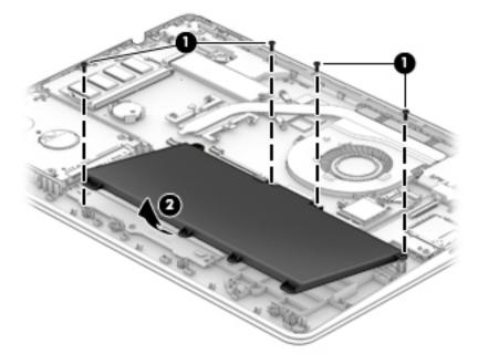
Reverse this procedure to install the battery.
