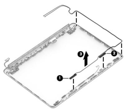
To remove the display/camera cable, disconnect the cable from the board at the bottom of the display (1) and the camera at the top of the display (2), and then remove the cable from the clips built into the side of the display enclosure (3).
