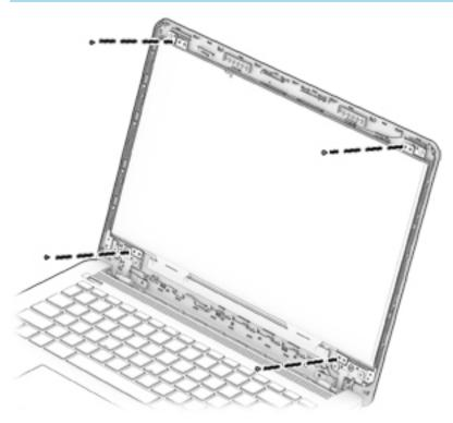
**b.** Rotate the display panel onto the keyboard **(1)** to gain access to the display cable connection on the back of the panel.
