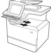
2. Open the left door. If jammed paper is visible inside the jam-access door, pull it straight out to remove it.
