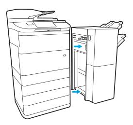
2. Move the finisher to a position where the finisher rear door is accessible, and then open the finisher rear door.
