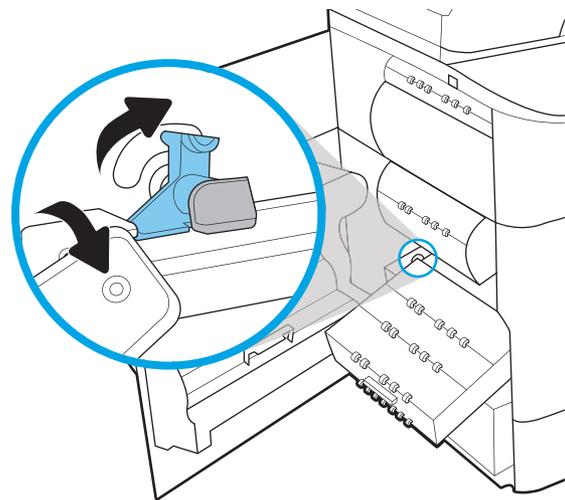
8. Push the service fluid container into the printer.
