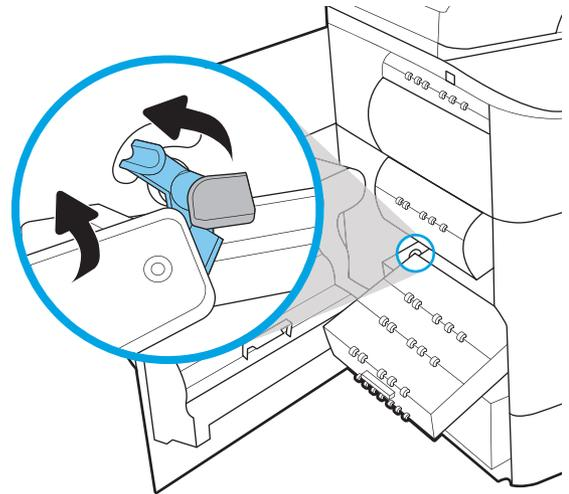
4. Remove the right side from the alignment track, and then remove the unit from the printer. Set the unit aside, upright, on a piece of paper to prevent spills.
