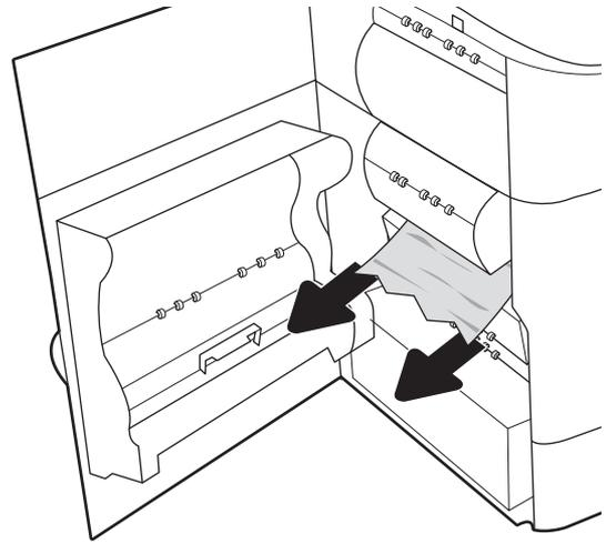
5. If no jammed paper is visible, pull the service fluid container out.
