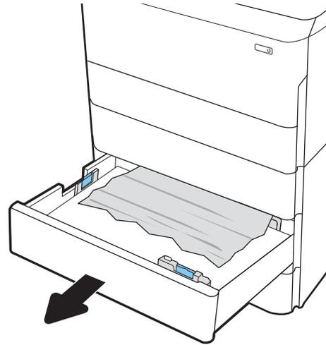
2. Remove the jammed paper from the feed rollers inside the printer. First pull the paper to the left, and then pull it forward to remove it.
