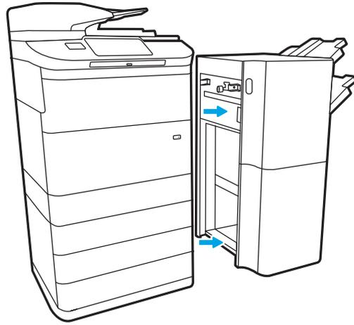
2. Move the finisher to a position where the finisher rear door is accessible, and then open the finisher rear door.
