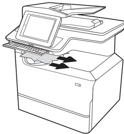
2. Open the left door. If jammed paper is visible inside the jam-access door, pull it straight out to remove it.
