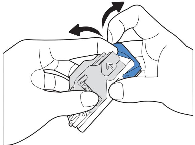
4. Close the lever at the back of the staple cartridge. Be sure that it snaps into place.
