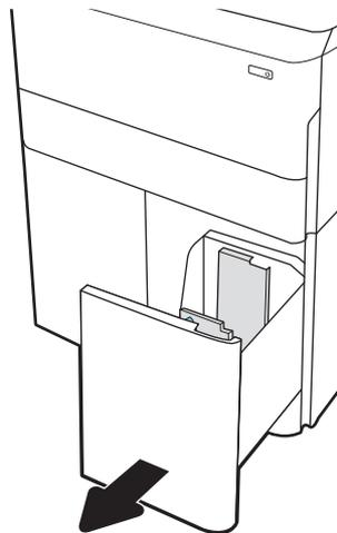
2. Adjust the paper-size guide to the correct position for the paper.
