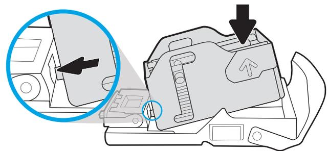
5. Insert the staple cartridge into the stapler and push on the colored handle until it snaps into place.
