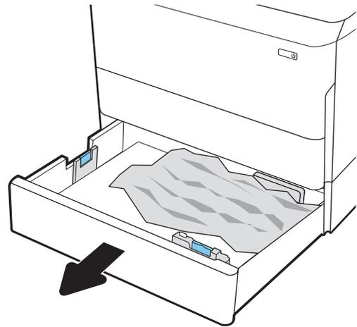
7. Remove the jammed paper from the feed rollers inside the printer. First pull the paper to the left, and then pull it forward to remove it.
