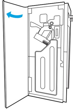
3. Turn the green wheel to bring the staple cartridge carriage toward you until it reaches its closest position, push down on the staple cartridge tab, and then slide the cartridge out of the finisher.
