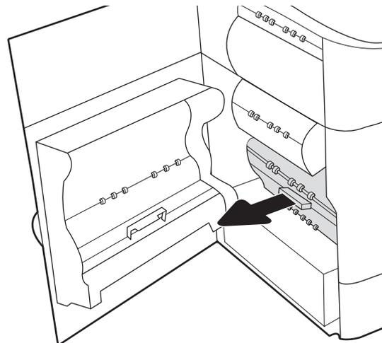
3. On the left side of the service fluid container, release the latch that holds the unit in the alignment track, and then remove the left side of the unit.
