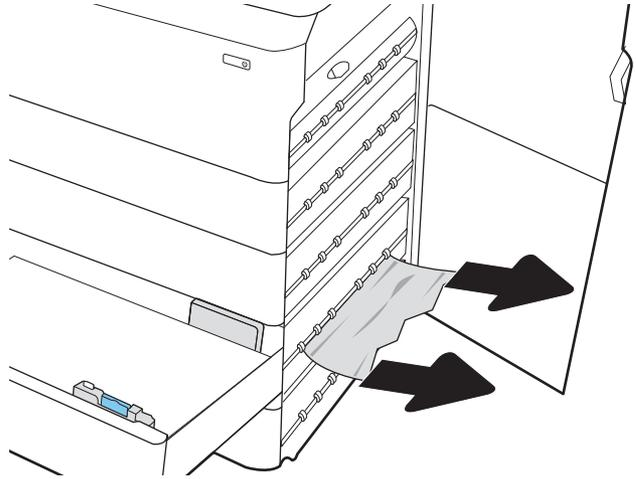
5. If no jammed paper is visible, remove the duplexer.
