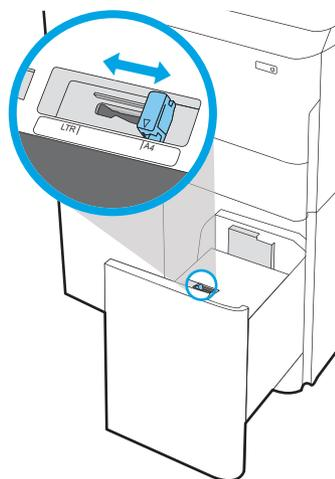
3. Load paper into the tray. Check the paper to verify the guides lightly touch the stack, but do not bend it.
