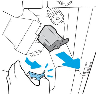
4. Lift up on the small lever at the back of the staple cartridge to separate the staple cartridge from the holder, and then remove any jammed staples.
