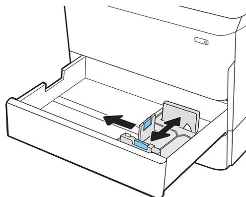
3. Load paper into the tray. Check the paper to verify that the guides touch the stack, but do not bend it. For information about how to orient the paper, see [Tray 2 and the 550-sheet trays paper orientation on page 41](#).
