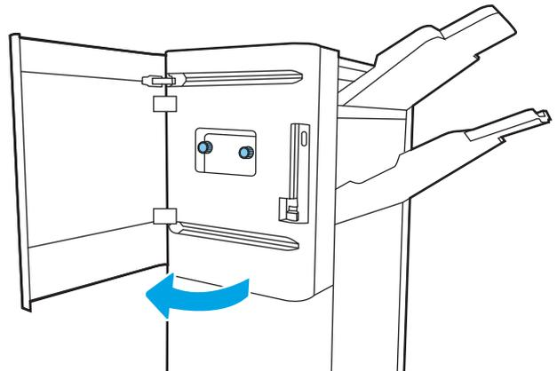
2. Rotate the green knobs, and then remove any jammed paper.
