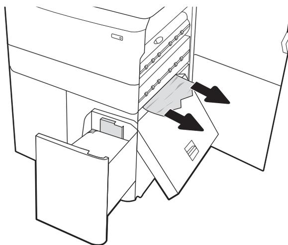
8. Use the green handle to open the top of the HCI jam cassette, and remove any jammed paper.
