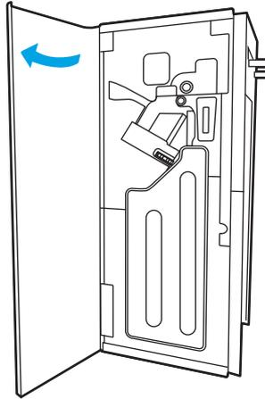
3. Rotate the green knobs, and then remove any jammed paper.
