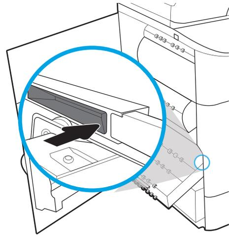
7. Insert the left end of the service fluid container into the alignment track, and then lock the latch that holds the unit in the track.
