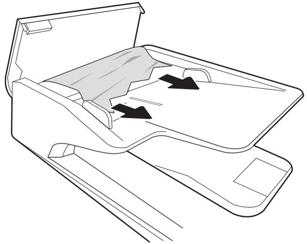
4. Lift the scanner lid and remove any jammed paper from the bottom of the scanner lid.
