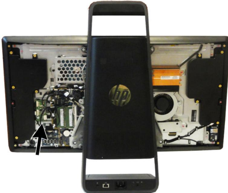
To remove the converter board:
