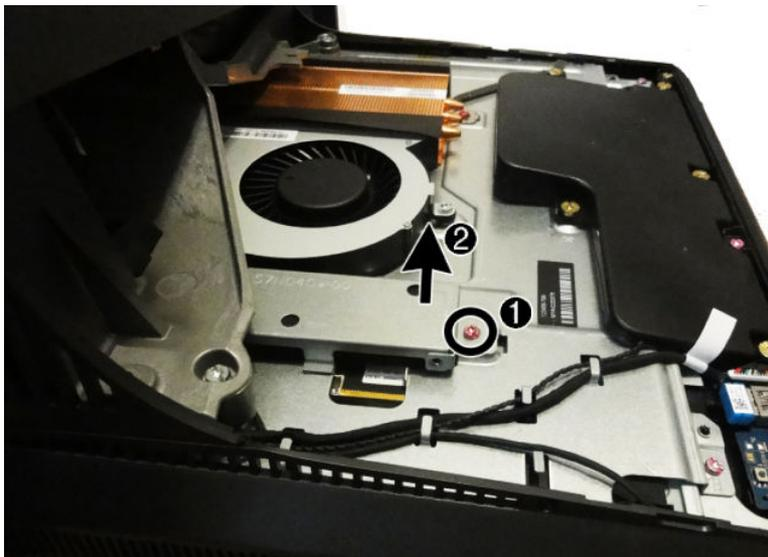
4. Remove the Phillips M2.0×3.0 screw **(1)** that secures the solid-state drive to the system board.
