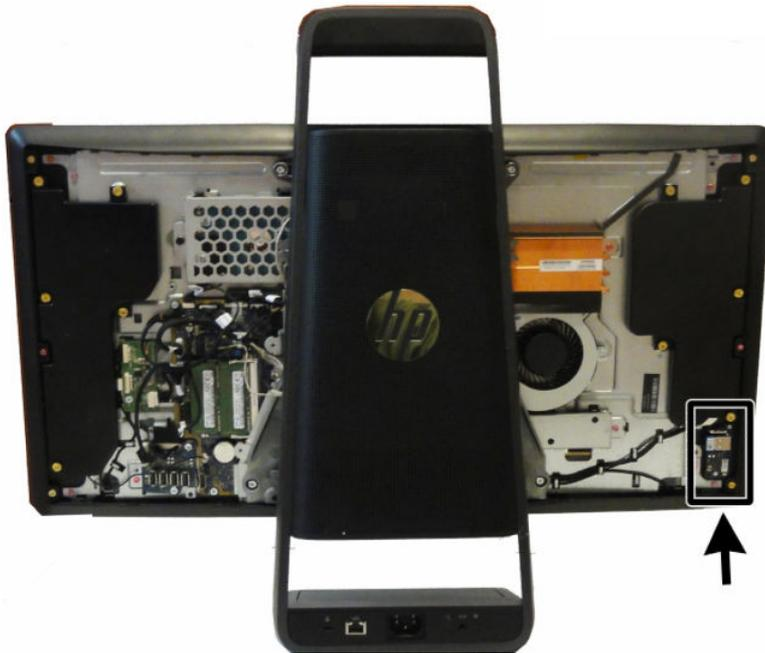
To remove the wireless USB/power button board:
