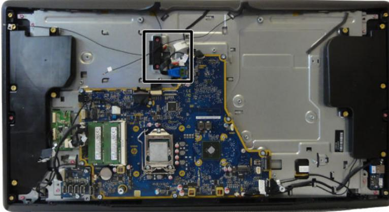
To remove the hard drive connector:
