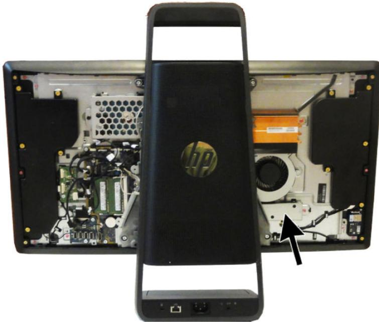
To remove the M.2 cover and solid-state drive:
