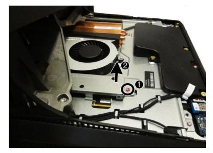
4. Remove the Phillips M2.0×3.0 screw (1) that secures the solid-state drive to the system board.
