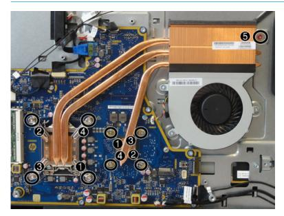
To replace the heat sink, reverse the removal procedures.
