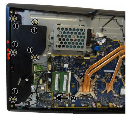
9. Remove the five Torx screws (1) that secure the left speaker to the computer.
