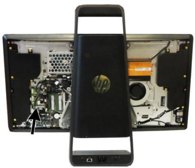
To remove the converter board:
