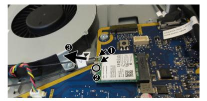
To install the WLAN module, reverse the removal procedures.
