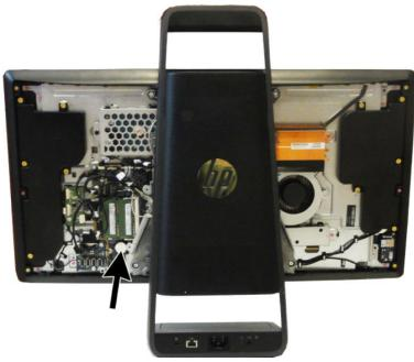
The battery that comes with the computer provides power to the real-time clock. When replacing the battery, use a battery equivalent to the battery originally installed in the computer. The computer comes with a 3-volt lithium coin cell battery.
