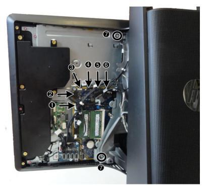
6. Remove the two screws from right side of the column.
