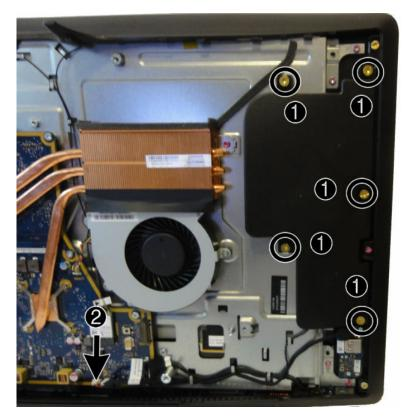
To install the speakers, reverse the removal procedures.
