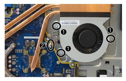
To install the fan assembly, reverse the removal procedures.
