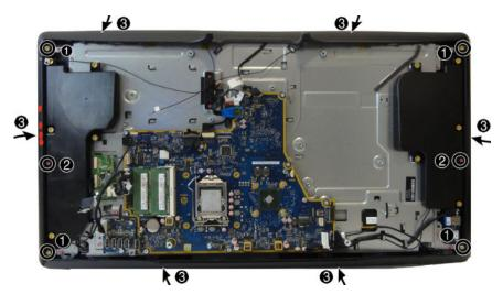
To install the outer plastic trim, reverse the removal procedures.
