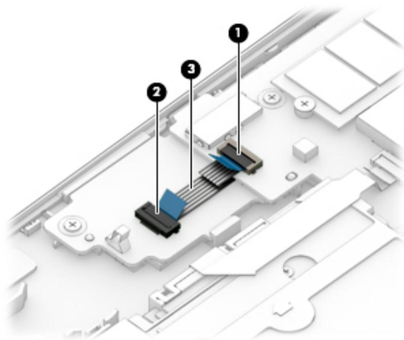
4. Remove the SD card board cable.
