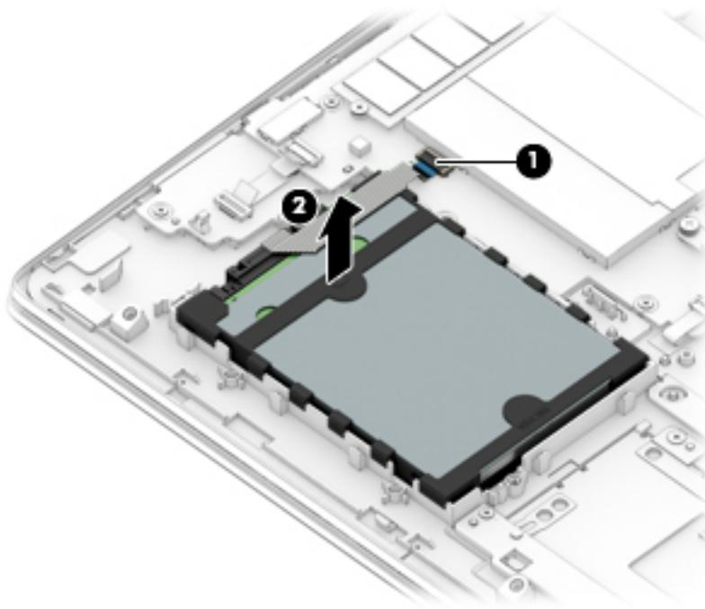
3. If it is necessary to disassemble the hard drive, remove the hard drive rubber sleeve (1) from the hard drive, and then disconnect the hard drive cable (2) from the hard drive.
