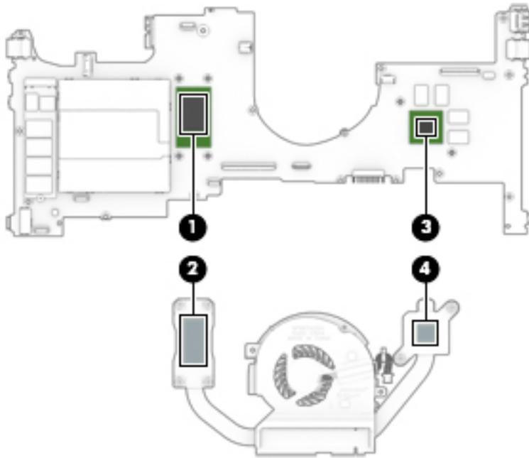
**On computer models equipped with a graphics subsystem with UMA memory:** Thermal paste is used on the processor (1) and the fan/heat sink assembly section (2) that services it.
