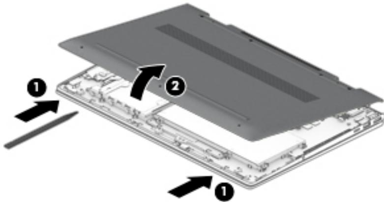
Reverse this procedure to install the bottom cover.
