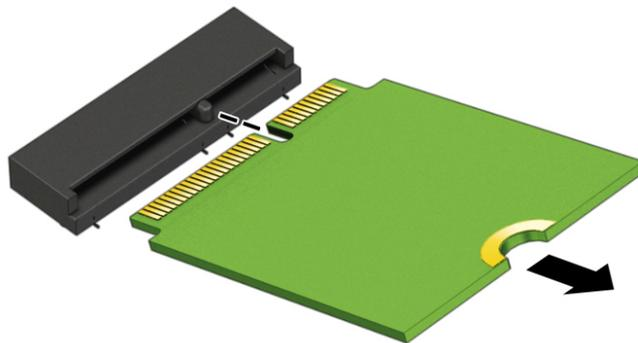
Reverse this procedure to install the WLAN module.
