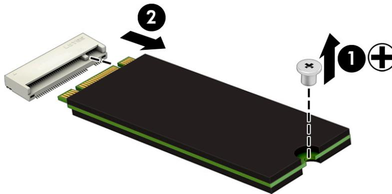
Reverse this procedure to reassemble and install the solid-state drive.
