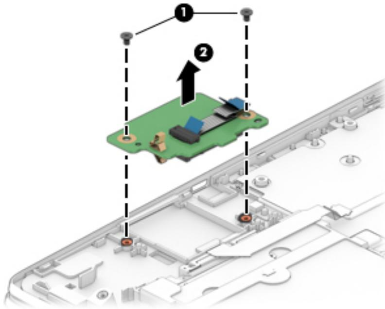
Reverse this procedure to install the SD card board.
