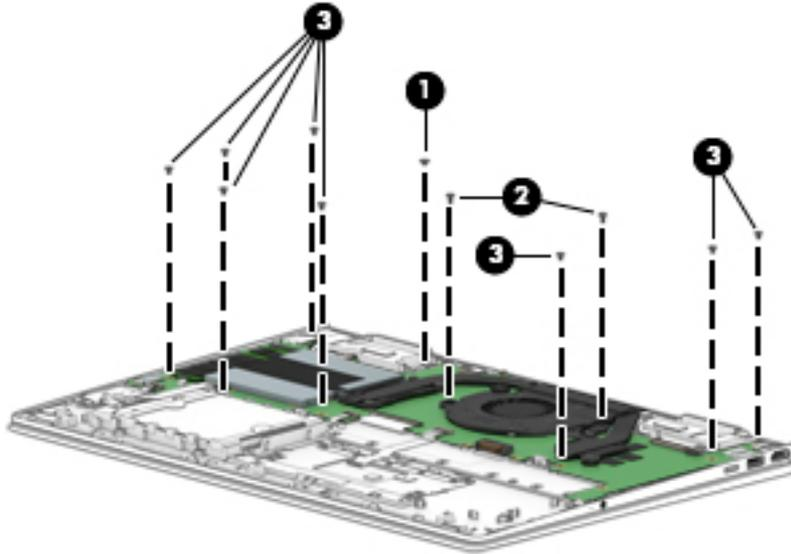
3. Lift the left side of the system board (1) until it rests at an angle.
