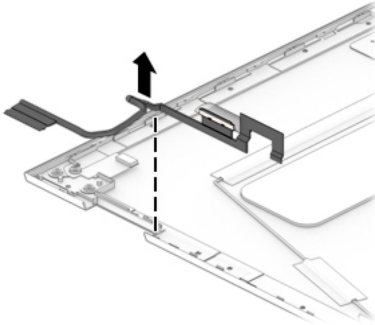
**13.** If it is necessary to replace the webcam/microphone module cable:
