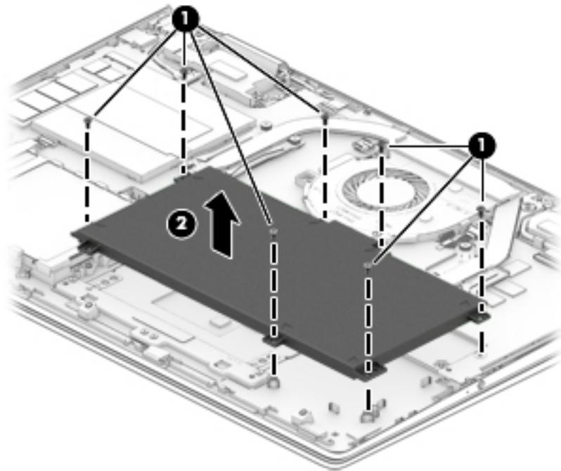
Reverse this procedure to install the battery.
