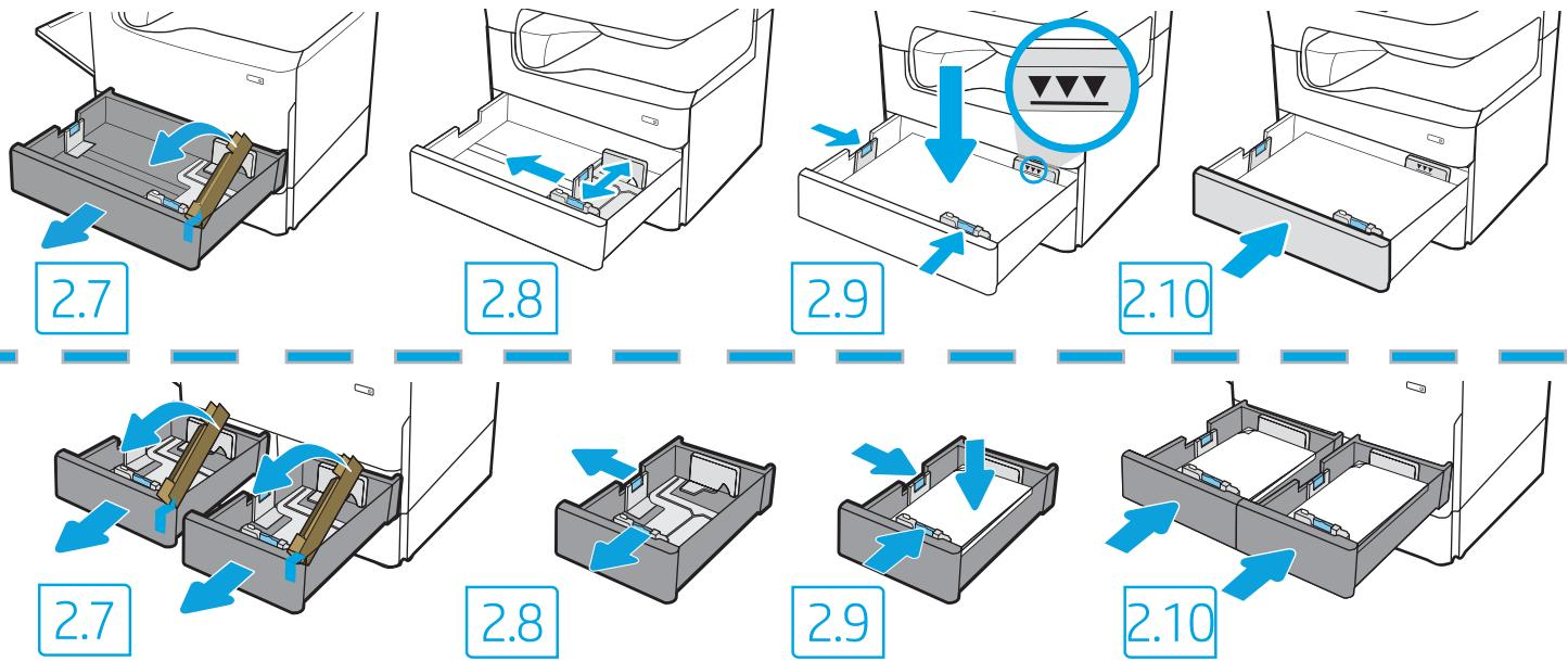
**EN** **CAUTION:** Use Letter/A4 paper in Tray 2 to initialize the printer. The printer will not initialize correctly with Tabloid/A3 paper loaded in Tray 2.
