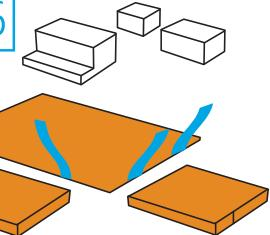
EN Remove all tape, packing material and orange restraints.
