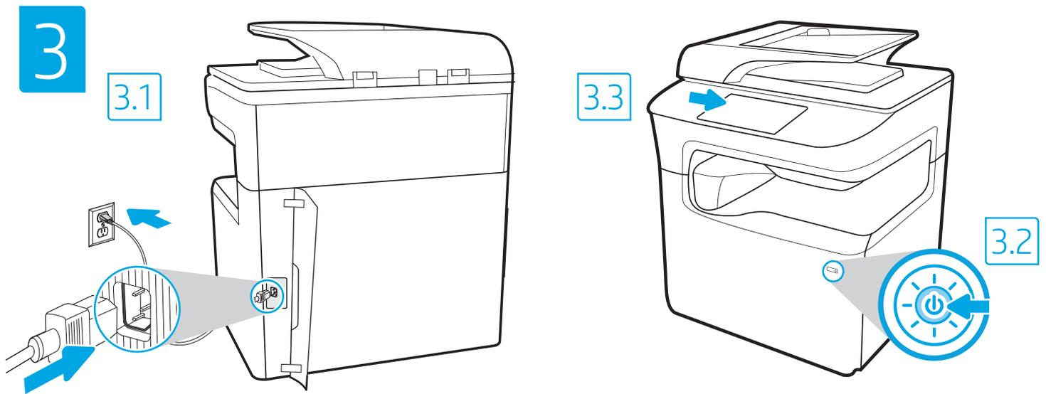
**EN** 3.1 Connect the power cable between the printer and a grounded AC outlet. 3.2 Turn on the printer. 3.3 On the Initial Setup screen, set the language, the location, the date/time format, and other features.
