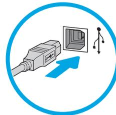
**EN Windows:** Do not connect the USB cable until prompted during the software installation in the next step. If the network cable was connected previously, proceed to the next section.
