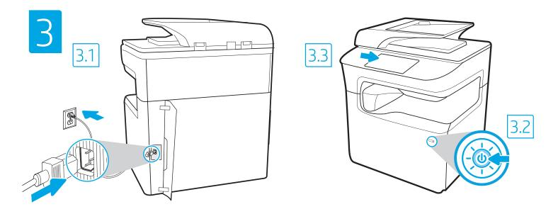
3.1 Connect the power cable between the printer and a grounded AC outlet. 3.2 Turn on the printer. 3.3 On the Initial Setup screen, set the language, the location, the date/time format, and other features.
