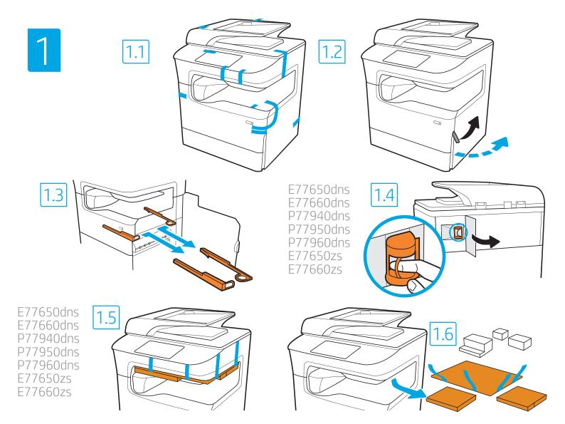
EN Remove all tape, packing material and orange restraints.
