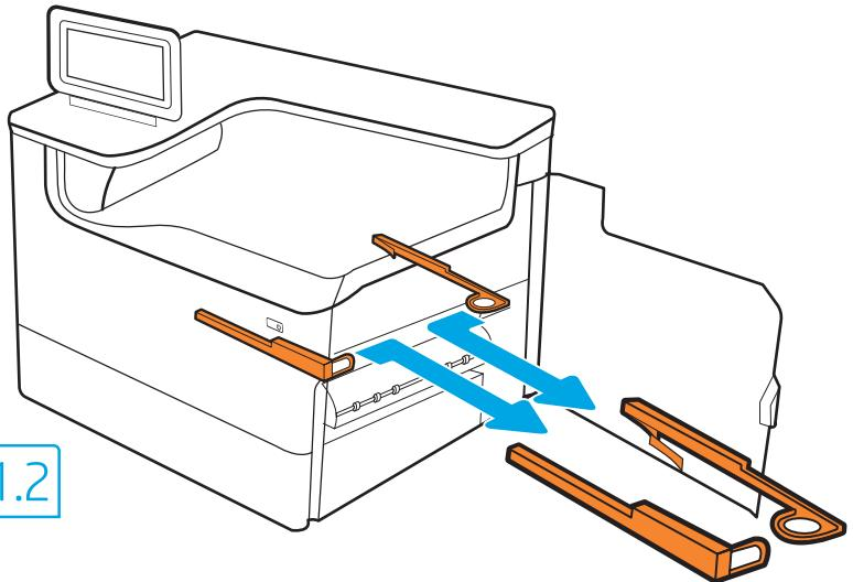
EN Remove all tape, packing material and orange restraints.
