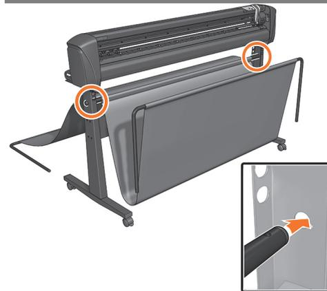
Insert the middle tube into the leg.
