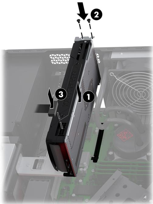
2. Place the bracket on the back of the graphics card (1), and then replace the screws (2).
