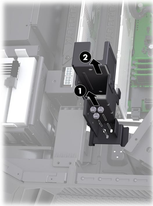
7. Remove the graphics card: Disconnect the power connector from the top of the card (1). Remove the two screws from the end of the card (2). Pull the PCIe socket latch (3), and then lift the graphics card up and out of the socket (4).
