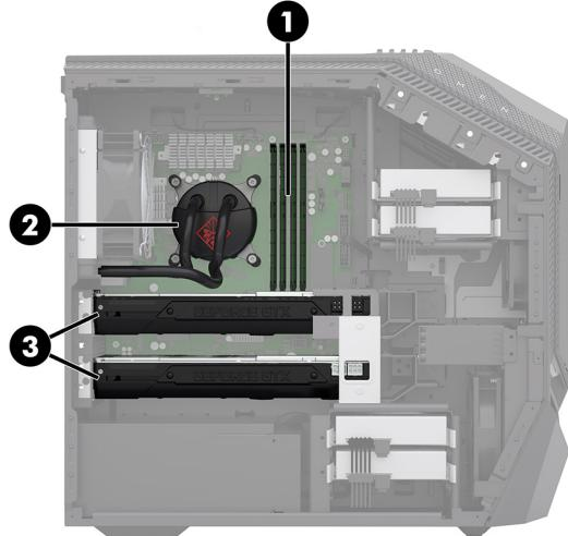
5. Remove the SLI bridge, if installed: Lift the bridge up from atop the graphics cards.
