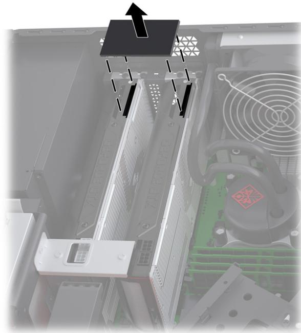
6. Remove the graphics card bracket: Remove the three screws (1), and then lift the bracket off the graphics card (2).
