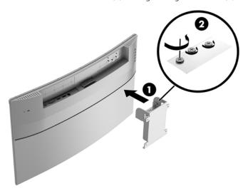
3. Secure the mounting plate to the wall or swing arm of your choice using the four screws included with the VESA mounting bracket.
