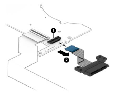
4. Remove the optical drive cable.
