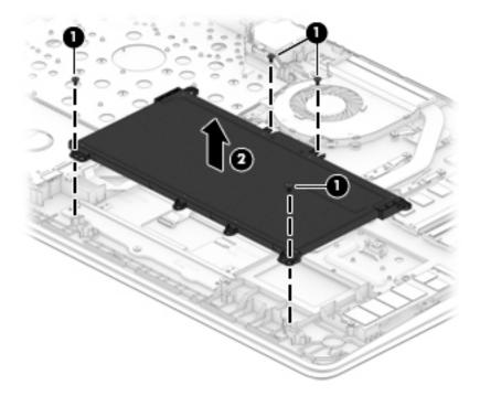
Reverse this procedure to install the battery.
