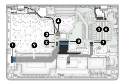
3. Remove the nine Phillips PM2.0×4.2 screws (1) that secure the system board to the keyboard/top cover.
