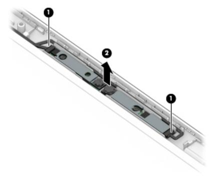
**d.** Remove the webcam/microphone module.
