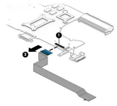
4. Remove the connector board cable.
