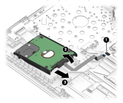
**4.** If it is necessary to disassemble the hard drive, remove the hard drive brackets **(1)** from the hard drive, and then disconnect the hard drive cable **(2)** from the hard drive.
