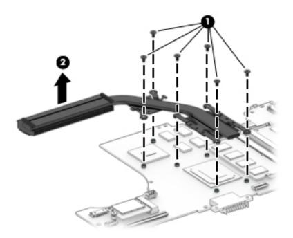
NOTE: The thermal material must be thoroughly cleaned from the surfaces of the heat sink and the system board components each time the heat sink is removed. Replacement thermal material is included with the heat sink and system board spare part kits.
