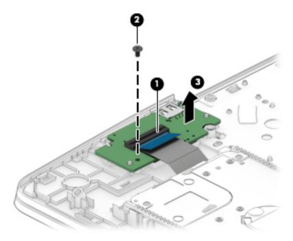
Reverse this procedure to install the connector board.
