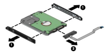
Reverse this procedure to reassemble and install the hard drive.
