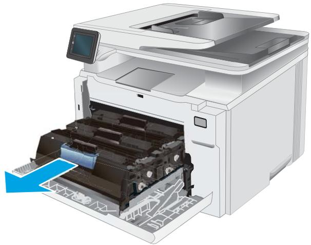
3. Grasp the handle on the toner cartridge, and then pull the toner cartridge straight up to remove it.
