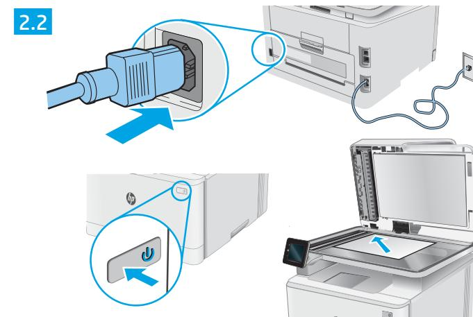
**EN** 1. Connect the phone cord for fax. A country/region specific adapter for the RJ11 telephone cord might be required to connect to the telephone jack.
