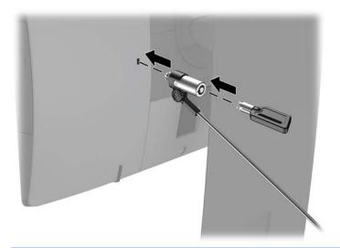
**CAUTION:** Use caution when adjusting the tilt, swivel, or height of the computer if a security cable is installed. The cable or the lock may interfere with the adjustment.
