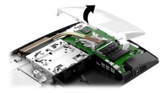
• If your computer model is a ProOne 400, use a flat blade or Torx screwdriver to remove the screws that secure the EMI shield and lift the shield off the computer.
