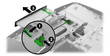
4. Pull the green latch off the optical disc drive.
