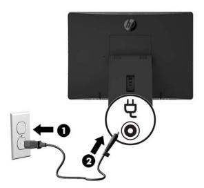
• Connect one end of the power cord to the AC adapter (1) and the other end to a grounded AC outlet (2), and then connect the AC adapter to the computer (3).
