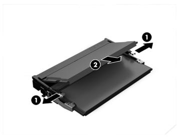
5. Slide the new memory module into the slot at approximately a 30° angle (1), then press the memory module down (2) so that the latches lock it in place.
