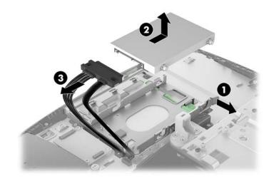
5. Remove the four mounting screws from the 2.5 inch hard drive. Be sure to keep the screws together with the blue rubber grommets to use to install a replacement drive.
