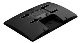
1. Press the supplied VESA trim plate onto the VESA opening until it snaps into place.
