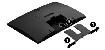
5. You may prevent access to internal components and ports by securing the rear port cover. Use a T15 tamper-resistant Torx screwdriver to screw the captive screw into the chassis.
