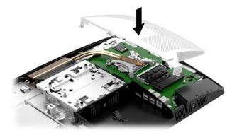
• If your computer model is a ProOne 400, place the EMI shield onto the chassis and use a flat blade or Torx screwdriver to fasten the screws to secure the EMI shield.
