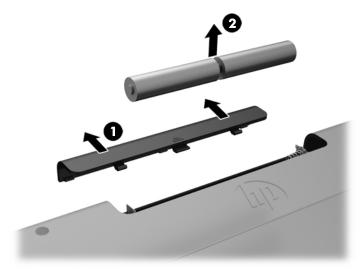
To remove batteries from the wireless mouse, remove the battery door on the underside of the mouse (1) and lift the batteries out of the battery compartment (2).
