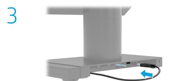
Connect the fingerprint reader USB cable to a USB Type-A port on the I/O connectivity base.
