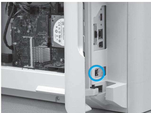
**EN** Before proceeding, take note of the location of the slot in the sheet metal where the fax telephone port must be installed.
