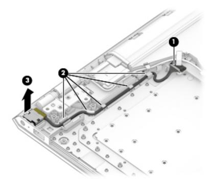
Reverse this procedure to install the power connector.
