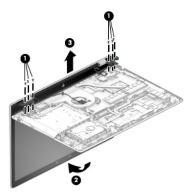
Reverse this procedure to replace the display assembly.
