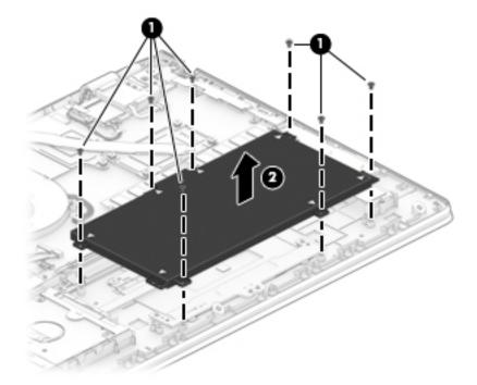
Reverse this procedure to install the battery.
