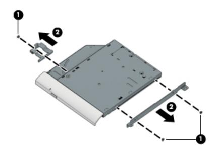
Reverse this procedure to install the optical drive.
