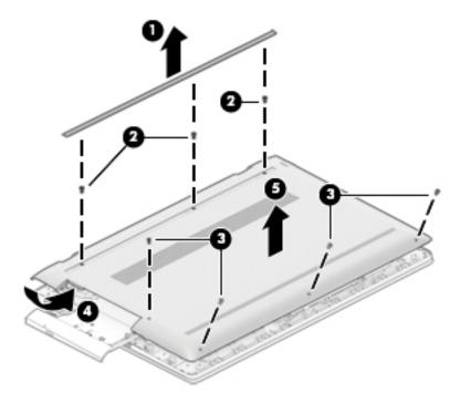
Reverse this procedure to install the base enclosure.
