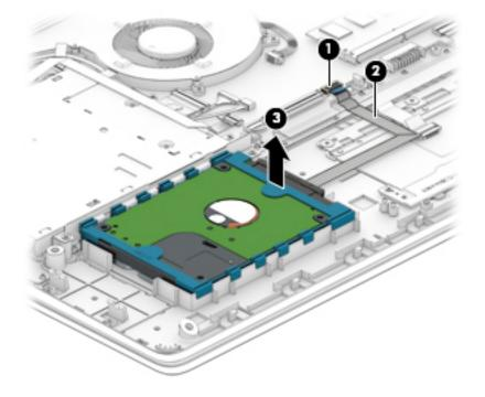
If it is necessary to disassemble the hard drive:
