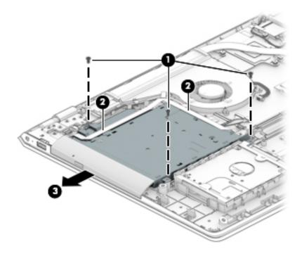
If it is necessary to remove the optical drive bracket:
