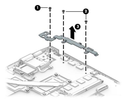
Remove the right input/output bracket:
