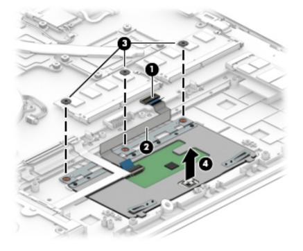
4. Disconnect the TouchPad cable from the system board (1) and the TouchPad (2), release the cable (3), and then lift the TouchPad cable (4) to remove it.
