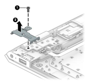
Reverse this procedure to install the input/output brackets.
