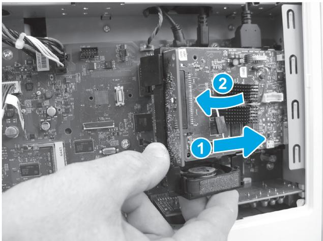
**EN** Insert the HDD cradle mounting tab in the slot in the sheet metal, slide the HDD toward the formatter cage (callout 1) to fully install the tab in the sheet metal, and then rotate the connector end (callout 2) of the HDD toward the formatter.
