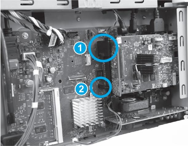
**EN** Make sure that the locking connector (callout 1) latches and that the standoff (callout 2) engages with the slot in the formatter (it might be necessary to pinch the retainer to engage it with the slot).
