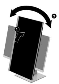
NOTE: To view information on the screen in portrait mode, you can install the HP Display Assistant software included on the software and documentation optical disc. The position of the OSD menu can also be rotated to portrait mode. To rotate the OSD menu, access the OSD menu by pressing the Menu button on the front bezel, select **OSD Control** from the menu, and then select **OSD Rotation**.
