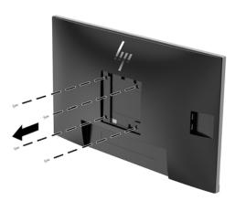
Install the mounting plate to the wall or swing arm of your choice using the four screws that were removed from the VESA holes on the rear of the display head.
