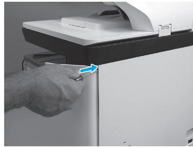
Open the right door, and then use a small flat-blade screwdriver to carefully push in against the latch to release it.
