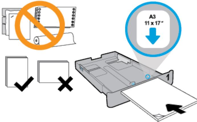
Make sure the stack of paper is aligned with the appropriate paper size lines on the front of the tray. Also, make sure the stack of paper does not exceed the stack height marking on the left edge of the tray.
