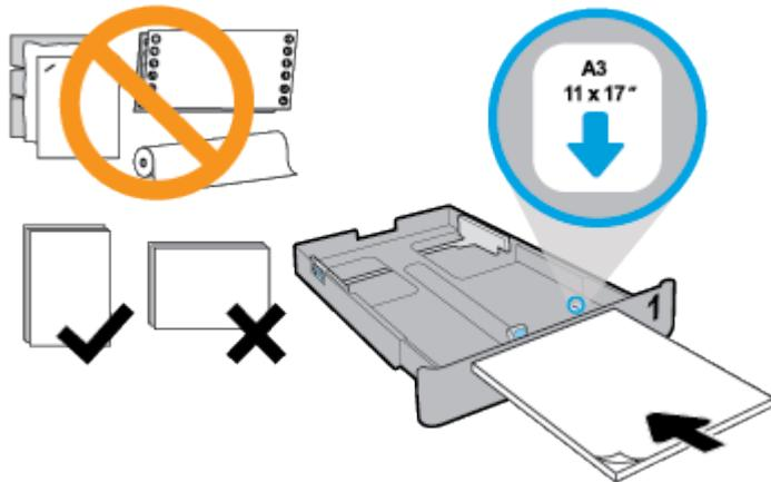
Make sure the stack of paper is aligned with the appropriate paper size lines on the front of the tray.
