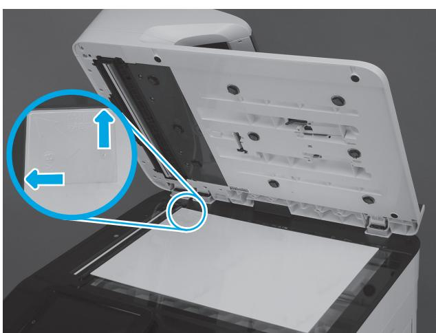
**EN** Place the reflector on the scanner glass. Make sure that the rear and left edge of the reflector are aligned with the rear and left edge of the scanner glass.
