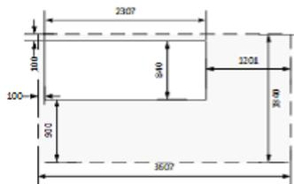
The space required for the cutter is illustrated below (measurements in millimeters):
