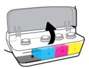
2. Remove the cap of the ink tank you plan to refill.
