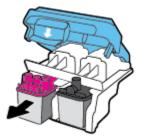
**e.** Check if there is a plug on top of the printhead or plastic tape on the printhead contacts. If there is, remove the plug from top of the printhead and the plastic tape from contacts.
