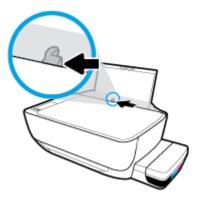
Insert one or more envelopes into the far-right side of the input tray and slide the stack of envelopes down until it stops.
