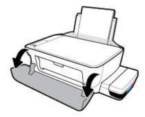
**b.** Open the printhead access door. Press and hold the **Black Copy** button for about three seconds, until the print carriage starts moving.
