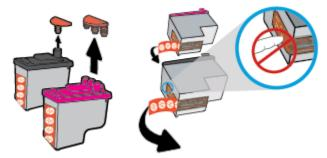
NOTE: Do not touch the electrical contacts on the printhead.
