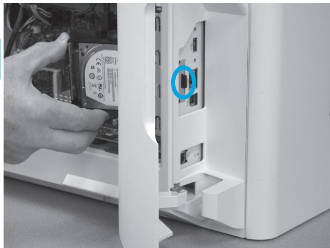
**EN** Before proceeding, take note of the location of the slot in the sheet metal where the HDD cradle mounting tab must be installed.
