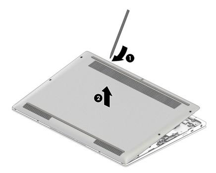
Reverse the removal procedures to install the bottom cover.
