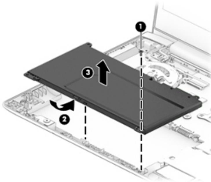
Reverse this procedure to install the battery.
