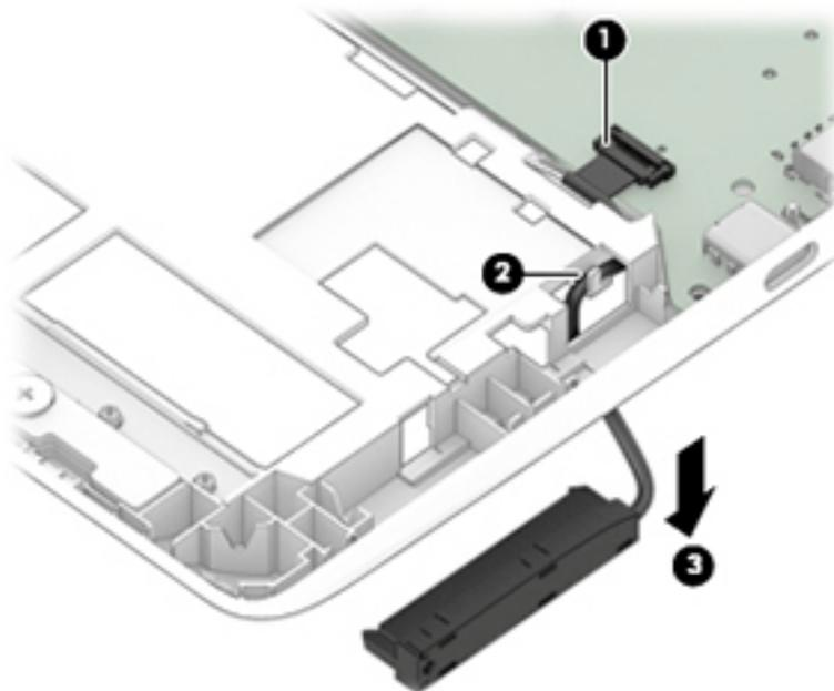
Reverse this procedure to install the hard drive cable.
