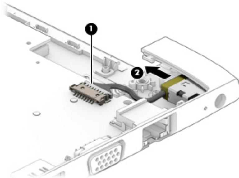
Reverse this procedure to install the power cable.
