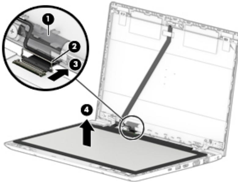
8. To remove the display enclosure, position the computer with the display enclosure lying on a flat surface and the computer upward at a 90 degree angle.
