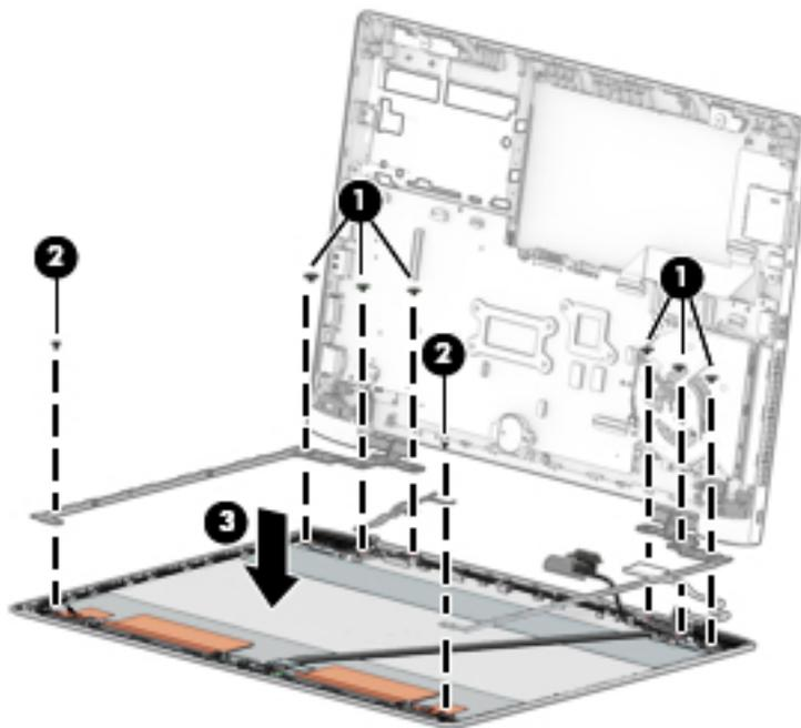
11. To remove the display hinges and brackets, remove the 4 Torx T8 2.5×4.0 screws (1) that secure the hinges to the computer, and then slide the hinges toward each other to remove them (2).
