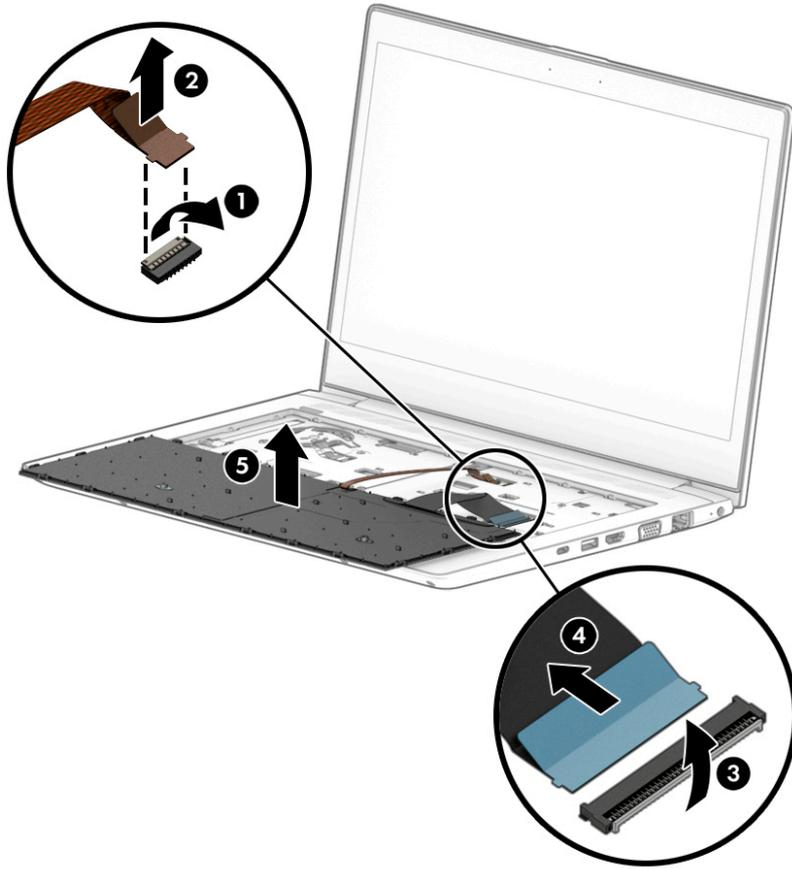
Reverse this procedure to install the keyboard.
