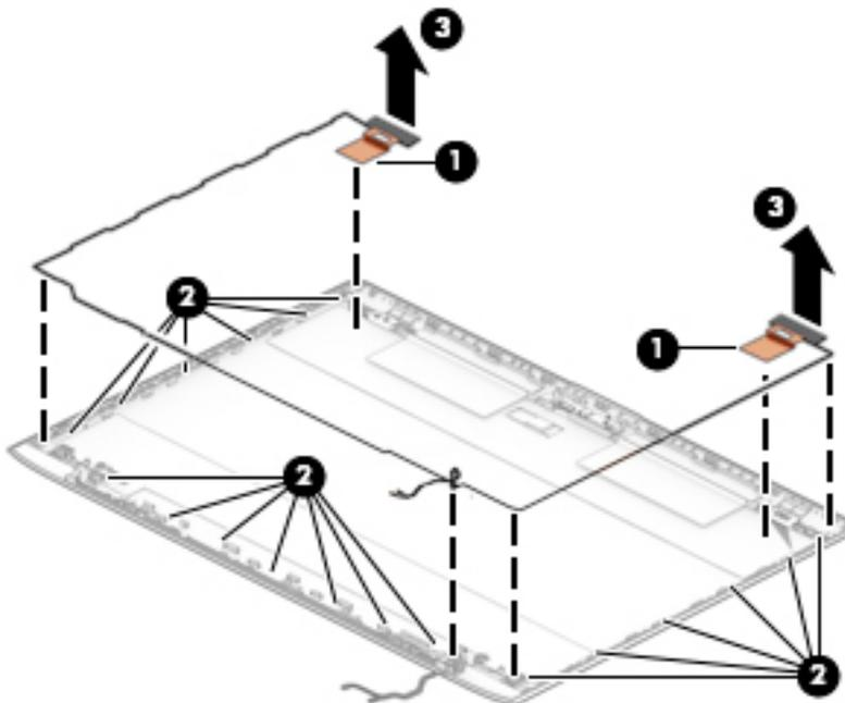
13. If it is necessary to remove or replace the HD camera, disconnect the cable from the camera (1), and then peel the camera module up to remove it from the adhesive that secures it to the enclosure (2).
