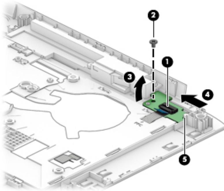
If you need to replace the cable, note the cable routing path inside of the top cover.
