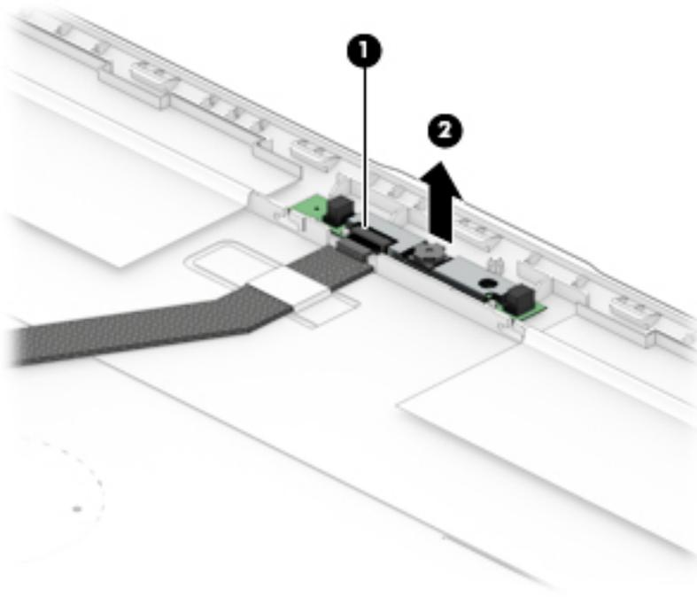
14. If it is necessary to remove or replace the HD display/camera cable, remove the cable from under the tab that secures it to the enclosure (1), and then remove the cable from the display enclosure (2).
