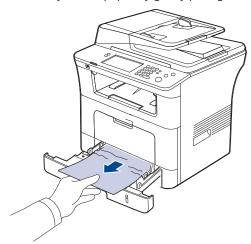
If the paper does not move when you pull, or if you do not see the paper in this area, check the fuser area around the toner cartridge. (See "Inside the machine" on page 4.)
