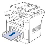
4. Squeeze the multi-purpose tray paper width guides and adjust them to the width of the paper. Do not force too much, or the paper will be bent, which will bent resulting in a paper jam or skew.
